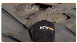
Put a waste oil container with at least 7 l capacity under the drainage hole.
