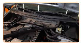
Unscrew the filter housing fastening bolts. Use Torx T20. Use a ratchet wrench.
