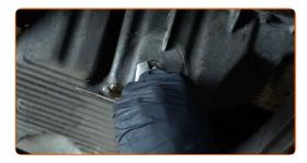
Screw in the new drainage plug and tighten it. Use a drive socket #19. Use a torque wrench. Tighten it to 25 Nm torque.
