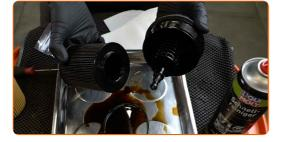
Clean the oil filter housing cap. Use all-purpose cleaning spray.
