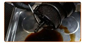
Detach the oil filter from the filter cover. Use a flat screwdriver.
