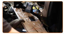
Remove the cabin filter housing cover. Use a Phillips screwdriver.
