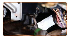
10 Remove the air distribution housing assembly.
