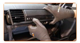
Unscrew the glove box fastening screws. Use a Phillips screwdriver. Use a flat screwdriver.
