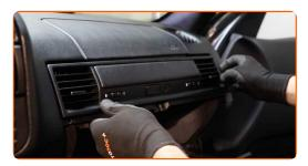
Screw the glove box fastening screws. Use a Phillips screwdriver.
