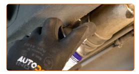
Loosen the fuel filter mounting. Use HEX No.H5. Use a ratchet wrench.
