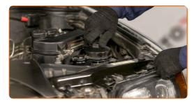
Use a drive socket #36. Use a torque wrench. Tighten it to 25 Nm torque.
