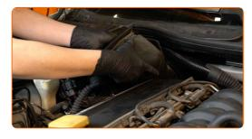
Install the engine cover and secure it.
