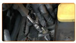
Tighten the ignition coil fasteners. Use a drive socket #10. Use a torque wrench. Tighten it to 11 nm torque.
