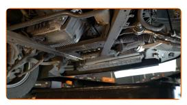
6 Clean the area of the oil pan drainage hole. Use a wire brush. Use all-purpose cleaning spray.
