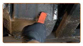
Unscrew the drain plug. Use a drive socket #17. Use a tap wrench.
