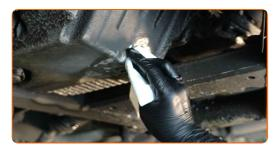
Screw in the new drainage plug and tighten it. Use a drive socket #17. Use a torque wrench. Tighten it to 25 Nm torque.
