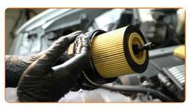
Install a new oil filter housing cover and tighten it. Use a drive socket #36. Use a torque wrench. Tighten it to 25 Nm torque.
