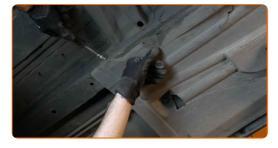
23 Install the clips of the underbody cover panel.
