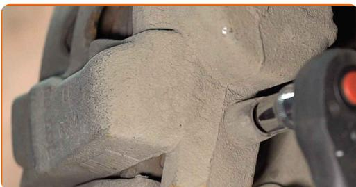
**11** Detach the brake caliper retaining spring. Use a crowbar.
