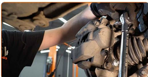
**52** Connect the brake pad wear sensor plug.
