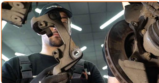
**17** Unscrew the brake disc fastening. Use HEX No.H4. Use a ratchet wrench.
