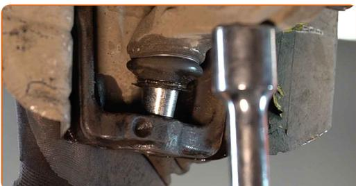
**38** Remove the support from under the arm.
