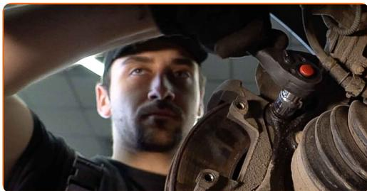
**16** Remove the caliper bracket.
