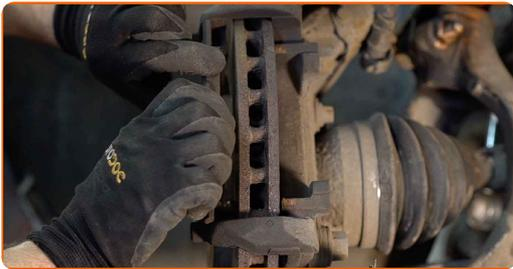
**14** Clean the brake caliper bracket fasteners. Use a wire brush. Use WD-40 spray.
