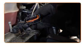
Plug in the ignition coil connector.
