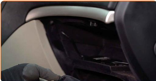
**3** Undo the glove box lining screw and remove the lining. Use a flat screwdriver. Use a Phillips screwdriver.
