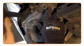
Screw in the fastening screws of the air filter cover. Use a drive socket #7. Use a ratchet wrench.
