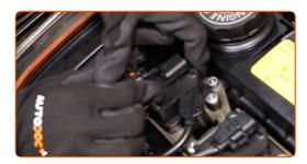
Unscrew the ignition coil bracket. Use Torx T40. Use a ratchet wrench.
