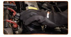
8 Tighten the oil filler cap.
