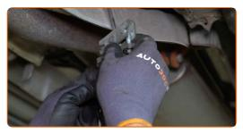
Clean the parking brake cable mounting seats. Use a wire brush. Use WD-40 spray.
