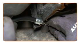
Secure the parking brake cable with the retaining clip. Use water pump pliers.
