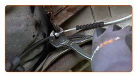
Attach the parking brake cable to the car body.
