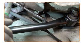
Clean the fastener of the parking brake cable. Use a wire brush. Use all-purpose cleaning spray.
