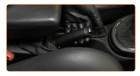
Loosen the parking brake cable. Use a combination spanner #13.
