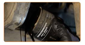
Replacement: engine oil and filter – ALFA ROMEO GTV (916C\_). Tip from AUTODOC:
