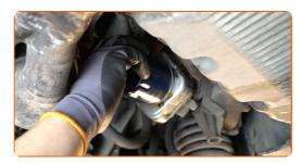
Tighten the oil filter. Remember to observe the recommended tightening torque. Use the 76-12F socket. Use a torque wrench. Tighten it to 18 Nm torque.
