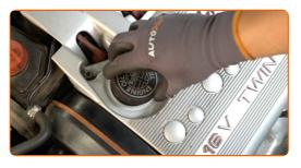
Tighten the oil filler cap.
