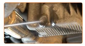
Unscrew the drain plug. Use Torx T50. Use a ratchet wrench.
