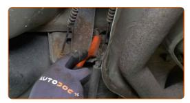
Remove the retaining clip of the parking brake cable. Use a crowbar. Use a hammer.
