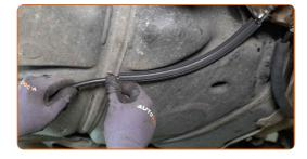
Screw in the parking brake cable fastener. Use a drive socket #10. Use a torque wrench. Tighten it to 6 Nm torque.
