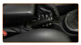
Loosen the parking brake cable. Use a combination spanner #13.
