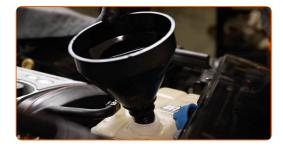
69 Pour coolant in the coolant reservoir.
