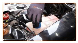
73 Screw on the coolant reservoir cap.
