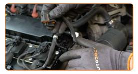
Disconnect the MAF sensor wiring. Use a flat screwdriver.
