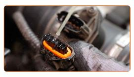
Attach the mass air flow sensor connector.
