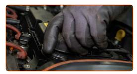
On the right side, detach the PCV valve hose from the engine cover. Use a flat screwdriver.
