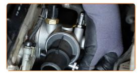
Tighten the thermostat housing fasteners. Use a drive socket #13. Use a torque wrench. Tighten it to 11 Nm torque.
