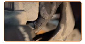
Disconnect the brake pad wear sensor plug.
