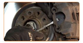
13 Remove the brake caliper.
