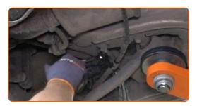
Detach the parking brake cable from the car body. Use a crowbar.
