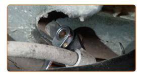
Detach the parking brake cable from the car body. Use a crowbar.
