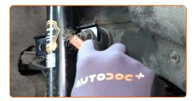
Unscrew the fastener connecting the stabilizer link to the shock strut. Use a combination spanner #17. Use HEX No.H5. Use a ratchet wrench.
