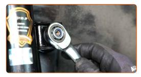
Tighten the fastener connecting the stabilizer link to the shock strut. Use a drive socket #17. Use a torque wrench. Tighten it to 55 Nm torque.
