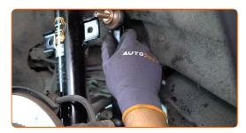
Tighten the stabiliser link fastener. Use a combination spanner #17. Use HEX No.H5. Use a ratchet wrench.
