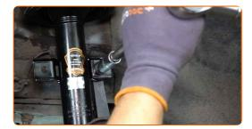
Tighten the fastener connecting the stabilizer link to the stabilizer bar. Use a drive socket #17. Use a torque wrench. Tighten it to 55 Nm torque.
