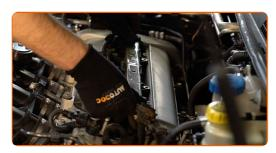
Tighten the ignition coil fastening. Use a drive socket #10. Use a torque wrench. Tighten it to 8 nm torque.
