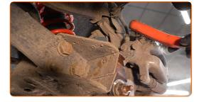
Unscrew the brake caliper fastening. Use a combination spanner #13. Use a combination spanner #15.
