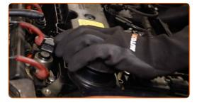
Tighten the oil filler cap.
