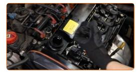
24 Install the engine cover and secure it.
