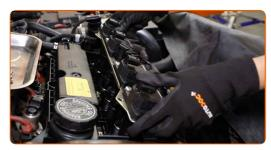
Tighten the ignition coil fastening. Use Torx T40. Use a torque wrench. Tighten it to 7 nm torque.
