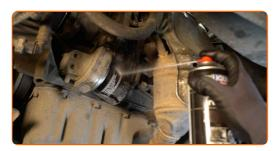
Unscrew the oil filter. Use the 76-12F socket. Use a ratchet wrench.
