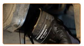
Replacement: engine oil and filter – ALFA ROMEO 166 (936). Tip from AUTODOC:
