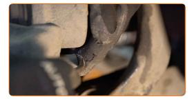
Disconnect the brake pad wear sensor plug.
