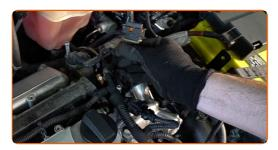
6 Unscrew the ignition coil bracket. Use a drive socket #10. Use a ratchet wrench.
