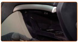
Undo the glove box lining screw and remove the lining. Use a flat screwdriver. Use a Phillips screwdriver.
