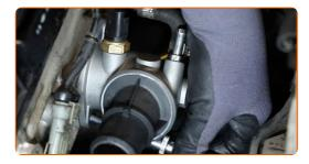
Tighten the thermostat housing fasteners. Use a drive socket #13. Use a torque wrench. Tighten it to 11 Nm torque.
