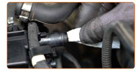
Detach the mass air flow sensor connector.
