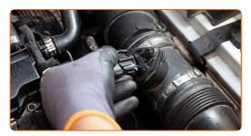
60 Connect the MAF sensor wiring.
