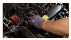
63 Install the engine cover and secure it.
