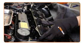
Tighten the ignition coil fastening. Use Torx T40. Use a torque wrench. Tighten it to 7 nm torque.
