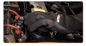
Tighten the oil filler cap.
