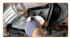
Screw in the new drainage plug and tighten it. Use Torx T50. Use a torque wrench. Tighten it to 20 nm torque.
