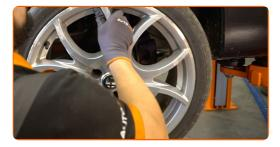
Detach the brake hose from the shock strut. Use a crowbar.
