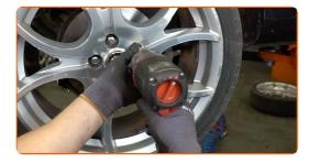
Lower the car and working in a cross order, tighten the wheel bolts. Use wheel impact socket #17. Use a torque wrench. Tighten it to 108 Nm torque.
