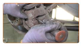
11 Remove the brake caliper. Use a crowbar.
