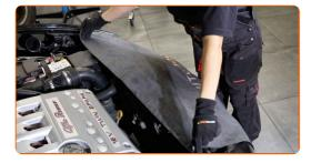
Unscrew the engine cover fastener. Use Torx T40. Use a ratchet wrench.
