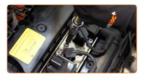
Take out the ignition coil from the spark plug well.
