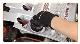
Screw in the engine cover fasteners. Use Torx T40. Use a ratchet wrench.
