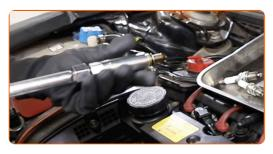
Apply a thin layer of a special high temperature anti-seize lubricant to the threads of the new spark plugs.
