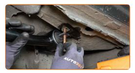
Screw the rear fastener connecting the control arm to the car body. Use a drive socket #15. Use a ratchet wrench.
