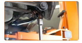
Tighten the rear fastener connecting the arm to the car body. Use a drive socket #15. Use a torque wrench. Tighten it to 68 nm torque.
