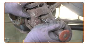
Remove the brake caliper. Use a crowbar.
