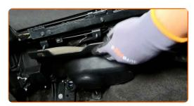
Screw in the fasteners of the passenger side kick panel. Use a drive socket #8. Use a ratchet wrench.
