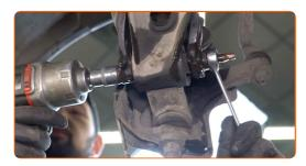
Remove the fastening bolt.
