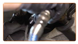
Remove the caliper bracket.
