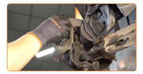
Tighten the brake caliper bracket. Use a drive socket #19. Use a torque wrench. Tighten it to 115 nm torque.
