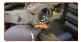
Unscrew the fastener that connects the wheel hub bearing to the steering knuckle. Use HEX No.H8. Use a ratchet wrench. Use a tap wrench.
