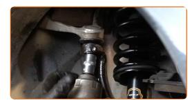
Detach the control arm. Use a ball joint puller.
