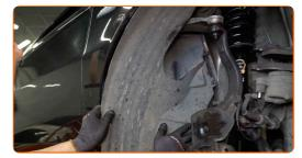
Install and tighten the wheel arch cover fasteners. Use a Phillips screwdriver.
