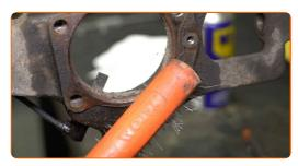
Pull the bearing inner race out of the wheel hub. Use a bush and bearing driver set. Use a bearing separator.
