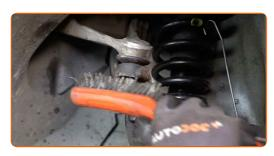
Unscrew the fastener that connects the suspension arm to the steering knuckle. Use a drive socket #17. Use a ratchet wrench.
