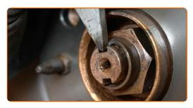
Treat all joints of the arm. Treat the steering knuckle fasteners. Use copper grease.
