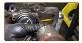
Tighten the fastener of the wheel hub bearing. Use HEX No.H8. Use a torque wrench. Tighten it to 76 Nm torque.
