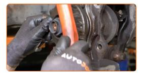
Install the brake disc.
