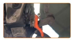
Unscrew the fastening bolt that connects the shock absorber fork with the lower control arm. Use a combination spanner #19. Use a drive socket #19. Use a ratchet wrench.
