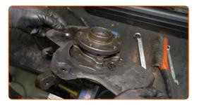
Screw in the fasteners of the brake disc cover. Use a drive socket #10. Use a ratchet wrench.
