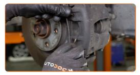
Tighten the drive shaft nut. Use a drive socket #38. Use a torque wrench. Tighten it to 177 Nm torque.
