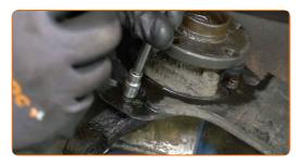
Remove the brake disc cover.
