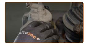
97 Install the brake caliper retaining spring. Use a crowbar.
