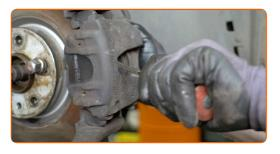
Remove the brake caliper.
