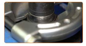
Treat the wheel hub bearing. Use copper grease.
