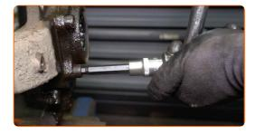
Loosen the vice and remove the steering knuckle.
