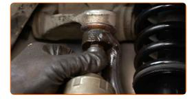
Detach the control arm. Use a ball joint puller.
