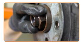
Unscrew the fastening bolt that connects the shock absorber fork with the lower control arm. Use a combination spanner #19. Use a drive socket #19. Use a ratchet wrench.
