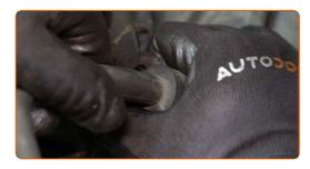
Disconnect the ABS sensor wiring.
