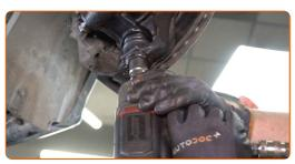
Tighten the fastener connecting the ball joint to the steering knuckle. Use a drive socket #24. Use a torque wrench. Tighten it to 90 nm torque.
