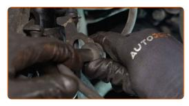
Install the brake hose retaining clip.
