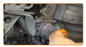
Unscrew and remove the wheel arch cover fasteners. Use a Phillips screwdriver.
