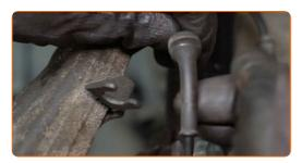
Detach the driveshaft from the steering knuckle.
