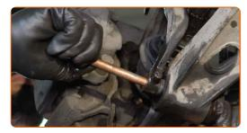
Unscrew the ball joint fastening to the steering knuckle. Use a drive socket #24. Use a ratchet wrench.
