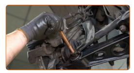
Screw in the fastener connecting the shock absorber fork to the lower control arm. Use a combination spanner #19. Use a drive socket #19. Use a ratchet wrench.
