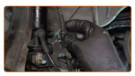
Fasten the brake hose on the strut.
