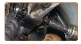
11 Remove the fastening bolt.
