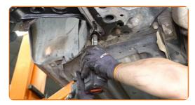
Tighten the fastener connecting the control arm to the subframe. Use a drive socket #15. Use a torque wrench. Tighten it to 71 nm torque.
