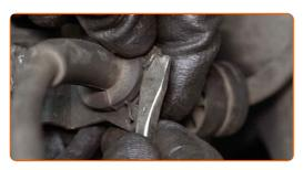
Detach the brake hose from the shock strut.
