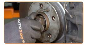
Screw the nut of the drive shaft. Use a drive socket #38. Use a ratchet wrench.
