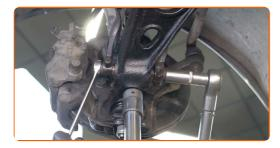
Remove the support from under the arm.
