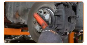
Loosen the fastener of the driveshaft. Use a drive socket #38. Use a tap wrench.
