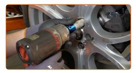
Lower the car and working in a cross order, tighten the wheel bolts. Use wheel impact socket #17. Use a torque wrench. Tighten it to 108 Nm torque.
