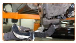
Clean the control arm fasteners. Use a wire brush. Use WD-40 spray.
