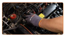
Install the engine cover and secure it.
