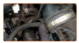
Unscrew the clamp and fasteners on the air filter intake pipe. Use a drive socket #7. Use a ratchet wrench.
