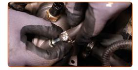
Secure the coolant hose clamp. Use clic-R collar pliers.
