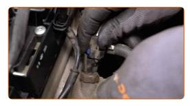
Loosen the coolant hose clamp. Use a flat screwdriver.
