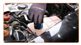
73 Screw on the coolant reservoir cap.
