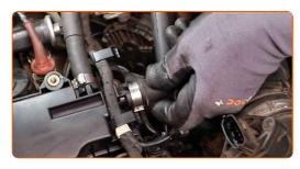
Treat the mass air flow sensor connector. Use dielectric grease.
