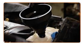
69 Pour coolant in the coolant reservoir.
