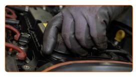
On the right side, detach the PCV valve hose from the engine cover. Use a flat screwdriver.
