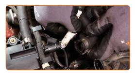
On the right side, attach the PCV valve hose to the engine cover. Use clic-R collar pliers.
