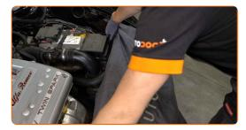
Unscrew the coolant reservoir cap.
