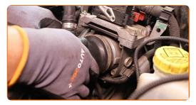
Tighten the clamp and fasteners on the air filter intake pipe. Use a drive socket #7. Use a ratchet wrench.
