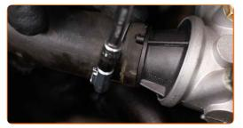
Treat the coolant temperature sensor connector. Use dielectric grease.
