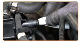
Detach the mass air flow sensor connector.
