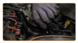
Tighten the oil filler cap.
