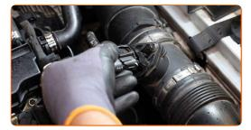
60 Connect the MAF sensor wiring.
