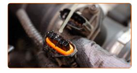
Attach the mass air flow sensor connector.
