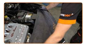
Remove the air filter housing retaining spring.
