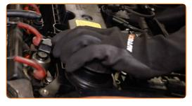
8 Tighten the oil filler cap.
