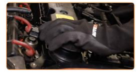
Tighten the oil filler cap.
