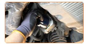
Tighten the oil filter. Remember to observe the recommended tightening torque. Use the 76-12F socket. Use a torque wrench. Tighten it to 18 Nm torque.
