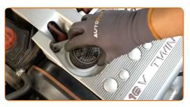
Tighten the oil filler cap.
