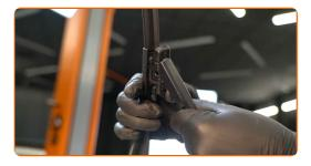
Remove the blade from the wiper arm.
