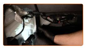
Screw in the fasteners of the cabin filter housing cover. Use Torx T25.
