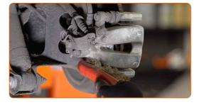
Unscrew the brake caliper fastening. Use a drive socket #13. Use a combination spanner #17. Use a ratchet wrench.
