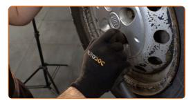
Lower the car and working in a cross order, tighten the wheel bolts. Use a torque wrench. Tighten it to 98 Nm torque.
