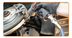
Screw the fastener connecting the control arm to the subframe. Use a combination spanner #18. Use a drive socket #18. Use a ratchet wrench.
