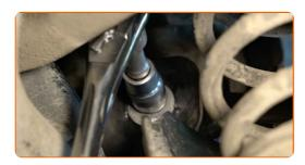
Tighten the arm fastening to the subframe. Use a drive socket #18. Use a torque wrench. Tighten it to 70 Nm torque.+180°
