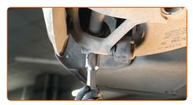
Unscrew the arm fastening from the subframe. Use a combination spanner #18. Use a drive socket #18. Use a ratchet wrench.
