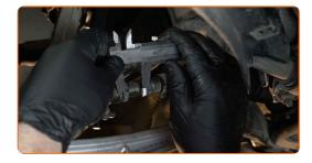
Loosen the lock nut securing the tie rod end to the tie rod. Use a combination spanner #24 (2 pieces).
