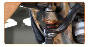
Screw on the fastening nut that connects the tie rod end to the steering knuckle. Use a combination spanner #21.
