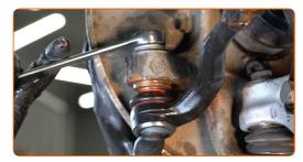
Tighten the tie rod end locknut. Use a combination spanner #24 (2 pieces). Use a torque wrench. Tighten it to 65 nm torque.
