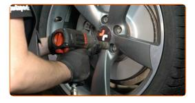
Lower the car and working in a cross order, tighten the wheel bolts. Use wheel impact socket #17. Use a torque wrench. Tighten it to 120 nm torque.
