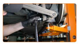
11 Remove the fastening bolt.
