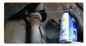
Unscrew the lower fastener of the shock absorber. Use a drive socket #21. Use a ratchet wrench.
