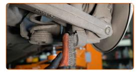
Unscrew and remove the wheel arch cover fasteners. Use a clip removal tool.
