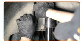
Install and tighten the wheel arch cover fasteners.
