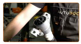
Screw the shock strut piston rod upper fastening. Use a shock absorber socket DDNº6. Use a drive socket #16. Use a torque wrench. Tighten it to 35 nm torque.
